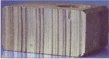
S9 • Tracking with hairlining and groves
