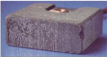
S15 • Eroded brush face
