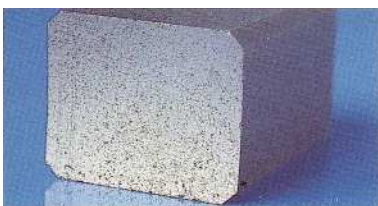
S3 • Slight porous sliding face
