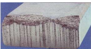
S23 • Broken edges
