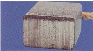
S13 • Burning edge of the leaving or trailing edge
