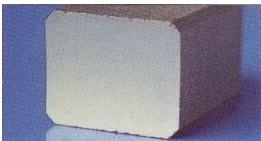
S1 • Dense, shining sliding face
