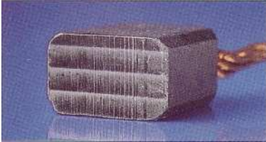
S17 • Lamination of sliding face
